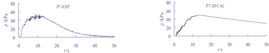
Fig.5 Response of pore pressure gauge P7 in test and calculation during earthquake
