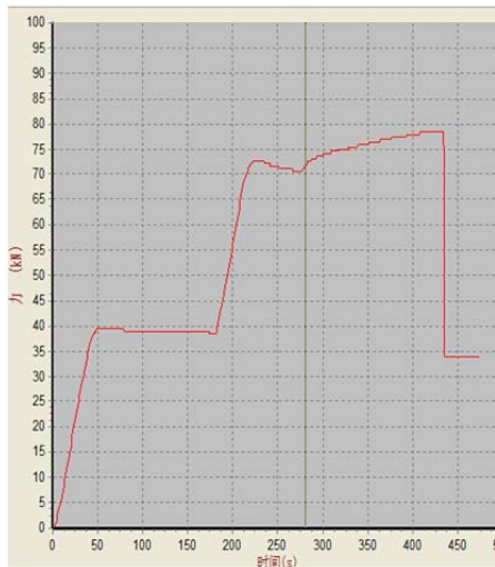
Fig 5 0mm steel core wire crimp pull Figure Fig 6 0mm steel core wire crimp pull Figure
