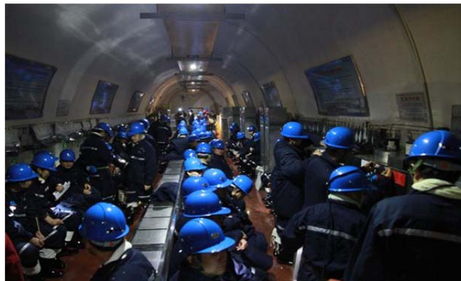
Fig. 1. Manned test of refuge chamber in the Mining Area I6 of Kong Village Coalmine
