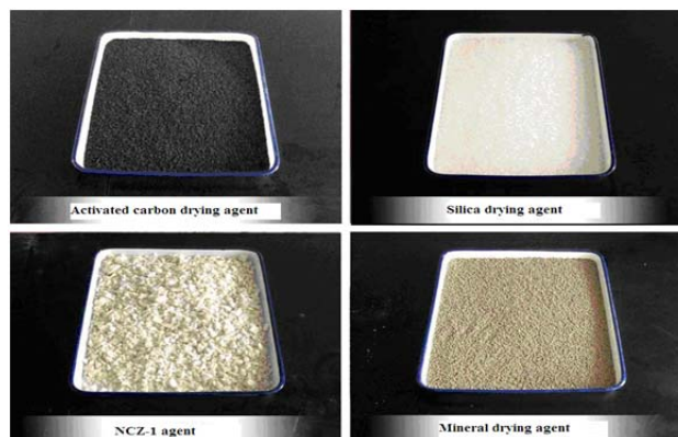
Fig. 10 Initial state of four dehumidizers on the trays
